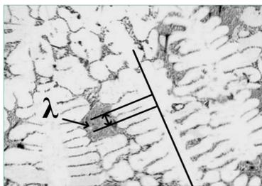
Fig. 1. Schematic of Secondary Dendrite Arm Spacing
