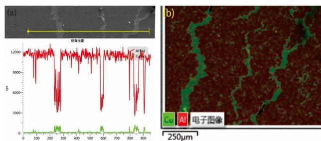
Fig. 4. Line and surface scanning analysis of linear segregation in ZL205A alloy
