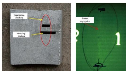
Fig. 1. Linear segregation of castings
