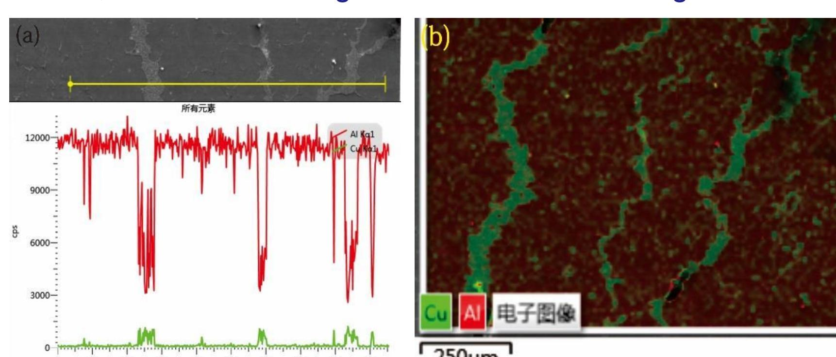
Fig. 4. Line and surface scanning analysis of linear segregation in ZL205A alloy
