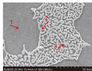
Fig. 3. SEM picture of linear segregation structure in ZL205A alloy
