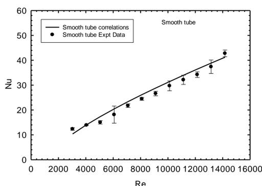
Fig. 3. Relationship between the Nu obtained from the experiment and the Nu according to the Gnielinski correlation for the smooth pipe.
