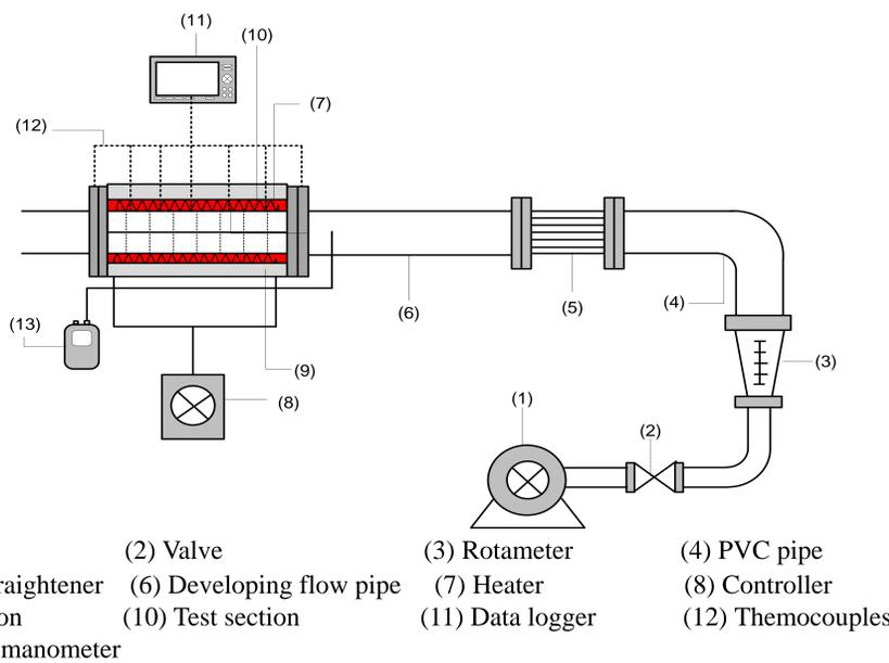
Fig. 1. Schematic diagram.
