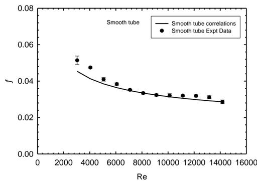
Fig. 4. Relationship between the f obtained from the experiment and the f calculated with Petukhov formula for the smooth pipe.
